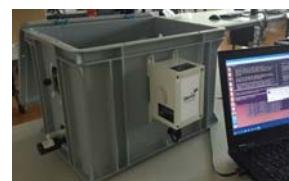
The prototype consists of two sensors boards protected by a box (see picture above) and is connected to a portable computer by USB. The communication architecture relies on POP-C++ objects and can be generic, independently of the actual sensors used; a driver must be available for each sensor.
